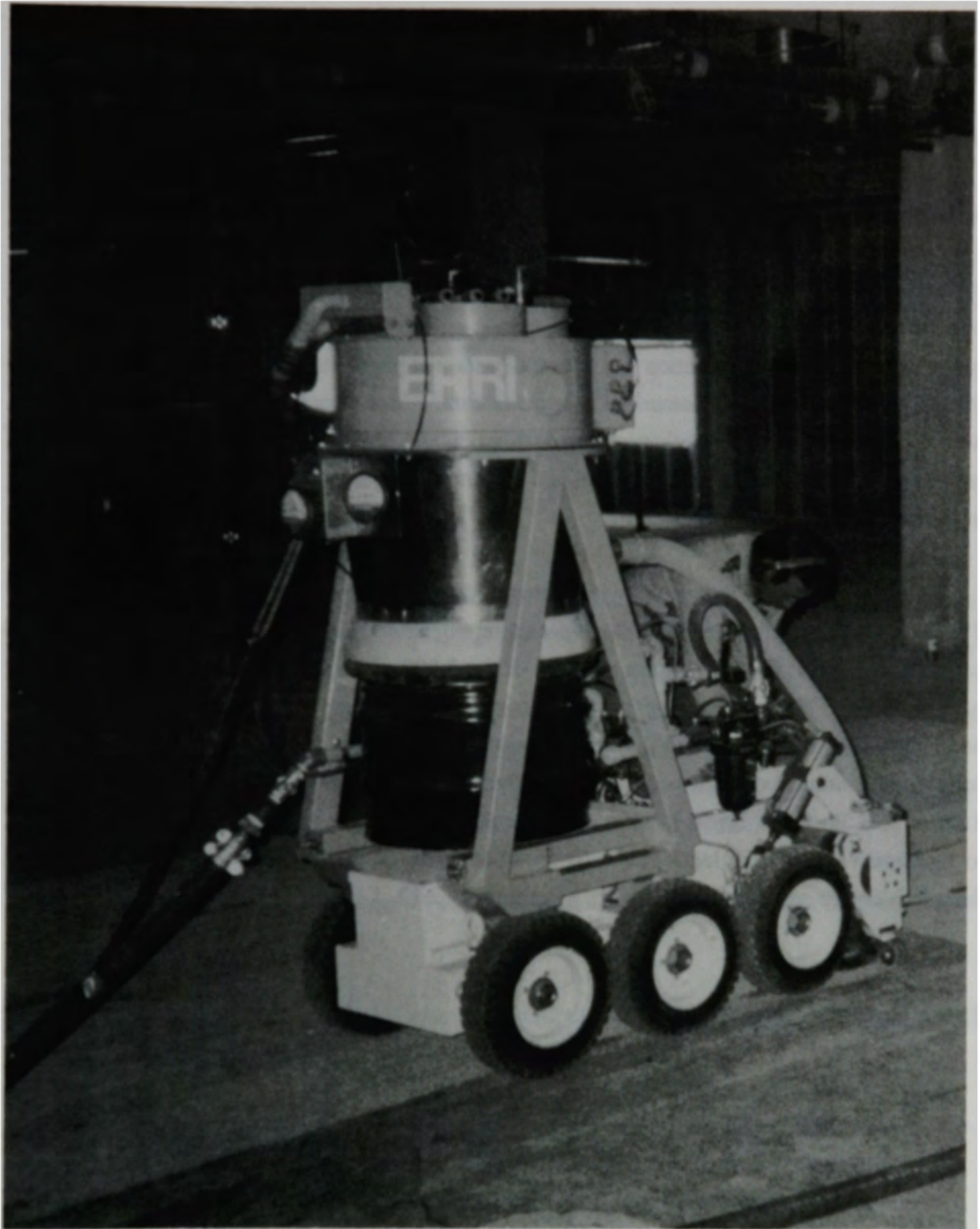
Figure 5. Remotely operated scabbler designed for use at TMI-2.
